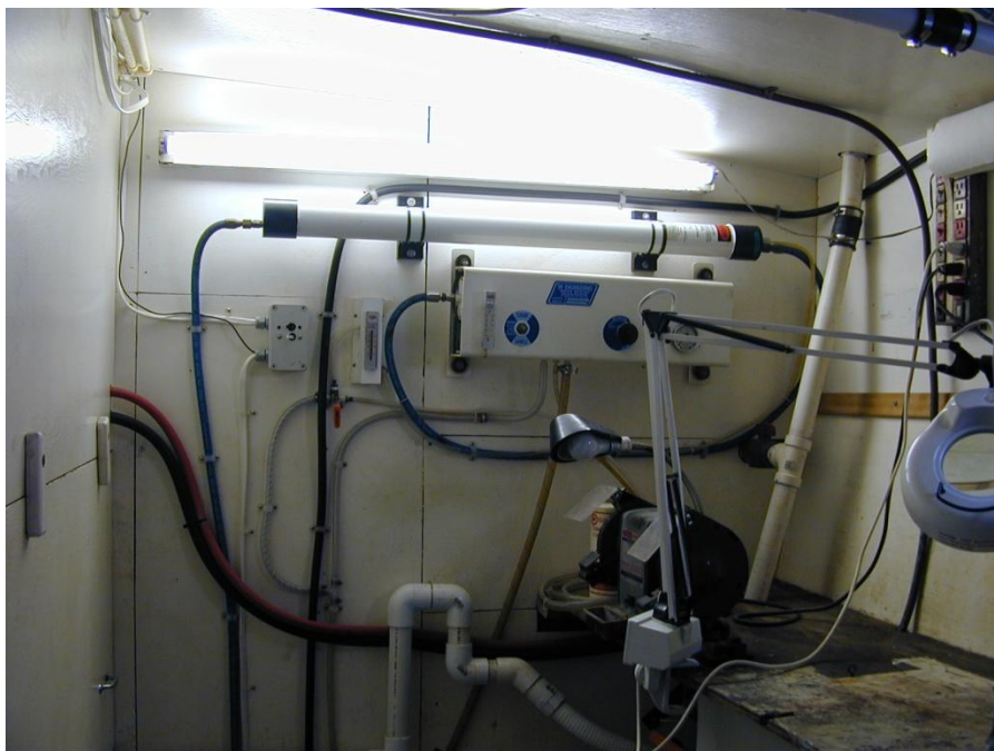
33 gph watermaker mounted on aft bulkhead in workshop area. Note port side engine access panel on left side of picture
